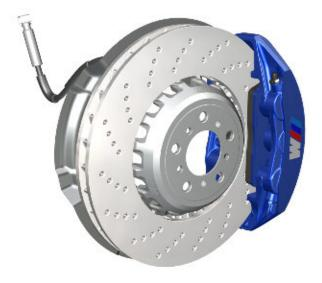
The front brakes are specific to the F12/F13 M6. It uses a large ventilated M Compound brake discs combined with a six-piston fixed calipers. In comparison to the F12/F13 650i, the diameter of the front brake disc @ 15.7 inches is 1.02 inches larger.
